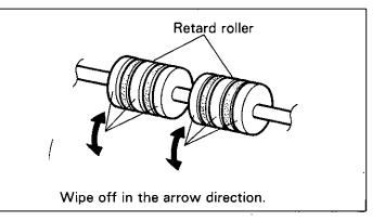
6 Use the accessory roller cleaning paper to wipe off the dirt on the surfaces of the six rubber carrier rollers and the five paper sensors.
